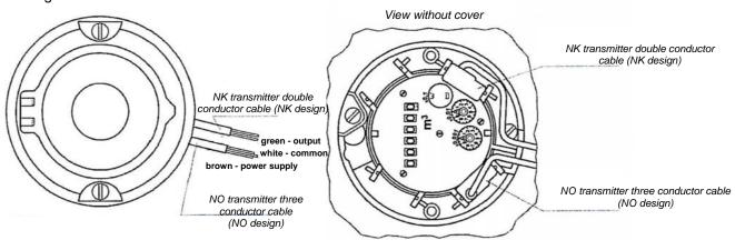
Warning: NKO design consists of a NK transmitter and a NO transmitter
